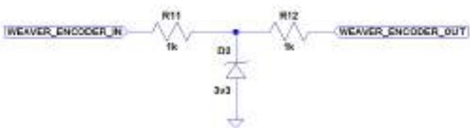
Fig. 10: Circuit of the Acquisition of Digital Signals
