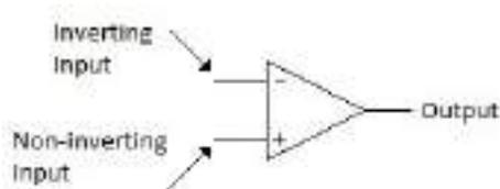
Fig. 2: Basic Operational Amplifier
