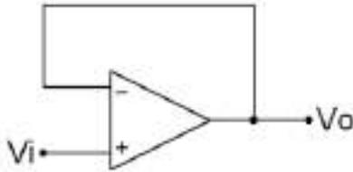
Fig. 6: Voltage Buffer Scheme
