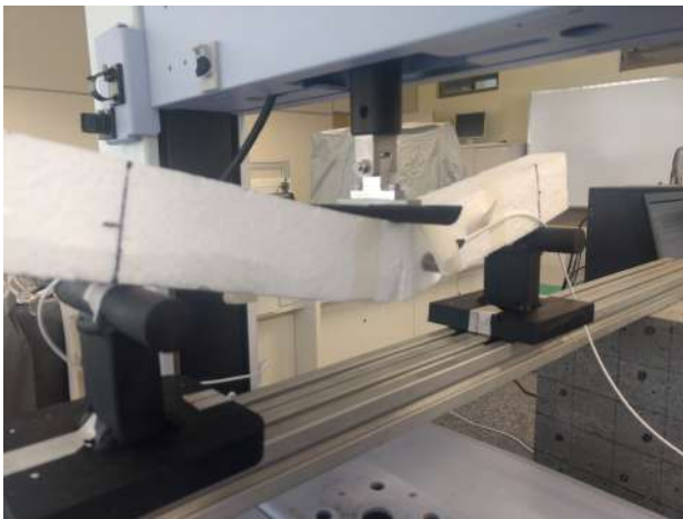
Fig. 10: Broken expanded polystyrene bar at the end of the rupture test.
